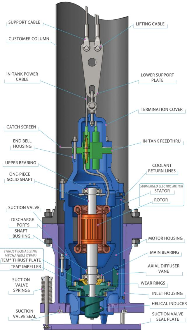
**Figure 1 Typical Pump in Column showing pump, suction valve & accessories**
