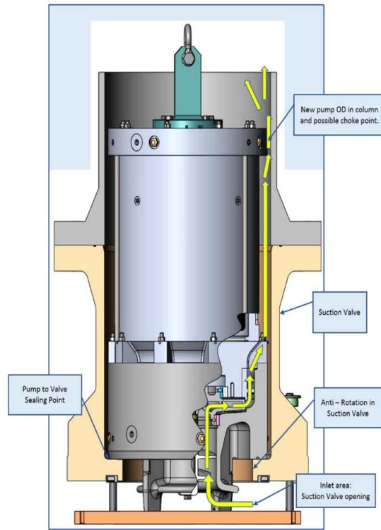
**Figure 2 Typical Pump in Column and Suction valve showing areas of detailed design study.**
